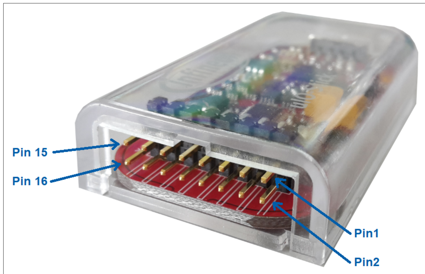
Figure 3 μIO-Stick Pin View
